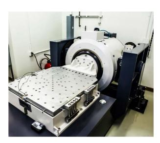
requirements. LST Series slip tables utilize V-groove bearings to guide the magnesium slip plate over an oil-film on a precision ground granite slab. Oil from an integral hydraulic power supply is dispersed through ports in the granite slab under the magnesium slip plate.
